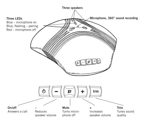
Konftel 60W is a conference unit for connecting to existing fixed system telephones, DECT telephones, cell phones or computers, with a cable or wireless connection via Bluetooth. Konftel 60W has a omnidirectional, highly-sensitive microphone and three speakers which, together with Konftel's OmniSound® provide optimal sound quality and maximum reduction of room echo, even when the person speaking is standing at a slight distance from the unit.
