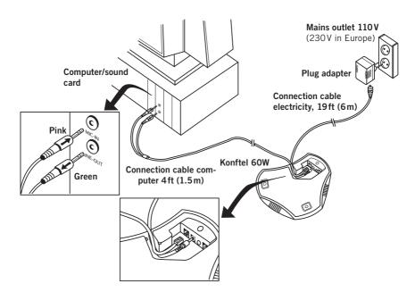
⇒ Connect Konftel 60W to the sound card using the accompanying Y-cable as per the picture.
